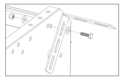
Using one 1/4" x 7/8" bolt, two 1/4" flat washers, and one 1/4" lock nut, bolt the L-mounting bracket to the rear pillar unit. There are existing holes in the rear pillar of the van that can be utilized. The picture shows a 46" high shelf installation. If installing a 43" high shelf, use the lower slot on the L-mounting bracket.
