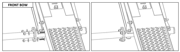
• Using three more 1/4" x 7/8" hex head screws, 1/4" washers, and 1/4" lock nuts, attach the opposite end of the torsion tube to the rear bow as shown below.
