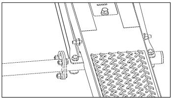
• Using three more 1/4" x 7/8" hex head screws, 1/4" washers, and 1/4" lock nuts, attach the opposite end of the torsion tube to the rear bow as shown below.
