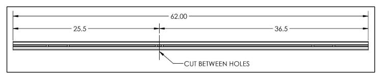
• The short rail is for the rear. The longer section is for the front.
