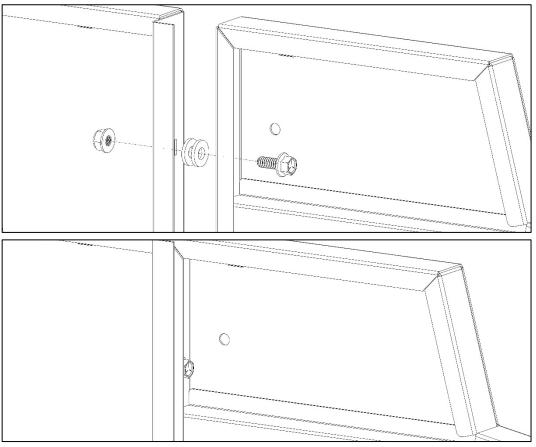
• Repeat 3 more times in the locations as shown below. Be sure to insert the washers between the panels if the door kit is being installed.
